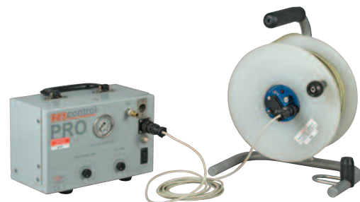
geocontrol PRO™ with optional draw-down control for low flow sampling
